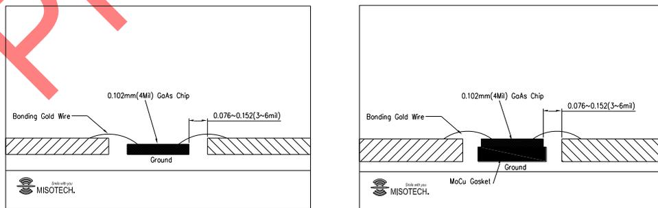
Note : Ceramic substrate should be close to the chip to shorten bonding wire.
