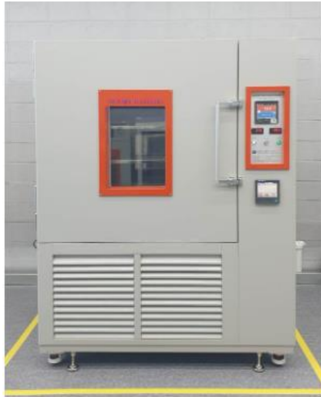
Constant Temp. & Humidity Chamber Woojin Tech Temperature range : -50 ~ +125deg Humidity : 30~95% 2 unit
